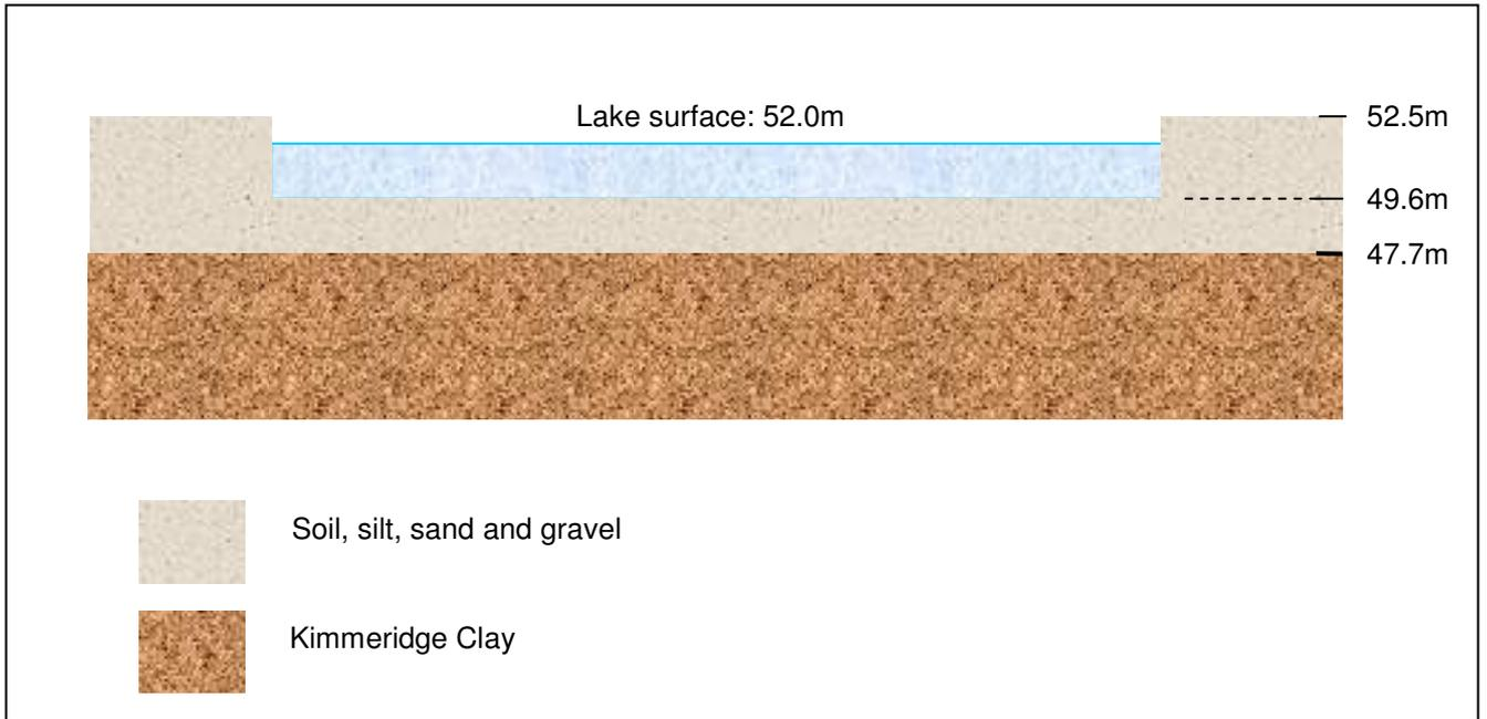
**Figure 2:** Schematic of vertical section of lake before filling, showing average levels (AOD) used in calculations. (Not to scale.)
